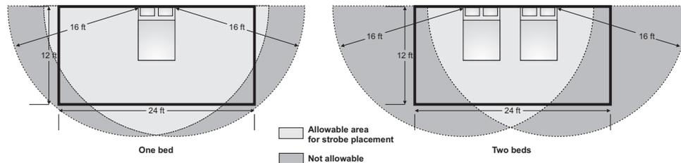
For the examples shown in Figure 3-12, the best placement for the strobe is on the wall directly opposite the bed.
