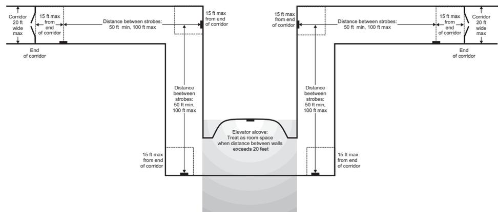
Distance between strobes should be no less than the prevailing requirement of 50 feet, and signals should not be placed more than 100 feet apart. Furthermore, the standards require that strobes be placed no less than 15 feet
