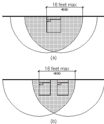
**702.3.6.3 Minimum Effective Intensity and Mounting Height.** Wall installed appliances located 24 inches (610 mm) minimum below the ceiling shall have a minimum effective intensity of 110 candela. Ceiling installed appliances and wall installed appliances located less than 24 inches (610 mm) below the ceiling shall have a minimum effective intensity of 177 candela.
