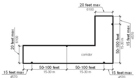
**702.3.5.1 Appliance Spacing.** Appliances shall be located 15 feet (4570 mm) maximum from each end of the corridor and shall be located 50 feet (15 m) minimum and 100 feet (30 m) maximum apart along the corridor. Interruptions to the concentrated viewing path by doors, elevation changes or other obstructions shall constitute the end of a corridor for purposes of this section.
