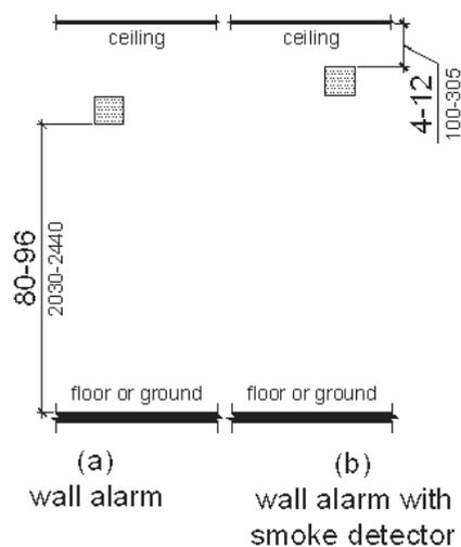
**EXCEPTION:** Wall installed appliances which are part of a smoke detector shall be located 4 inches (100 mm) minimum and 12 inches (305 mm) maximum below the ceiling measured to the top of the smoke detector.
