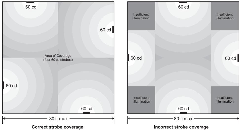
This configuration divides the room into squares, each one served by a different strobe as if the individual areas of coverage were independent spaces.<sup>34</sup> The same technique should be used for rectangular and irregular spaces as shown in Figure 3-6.
