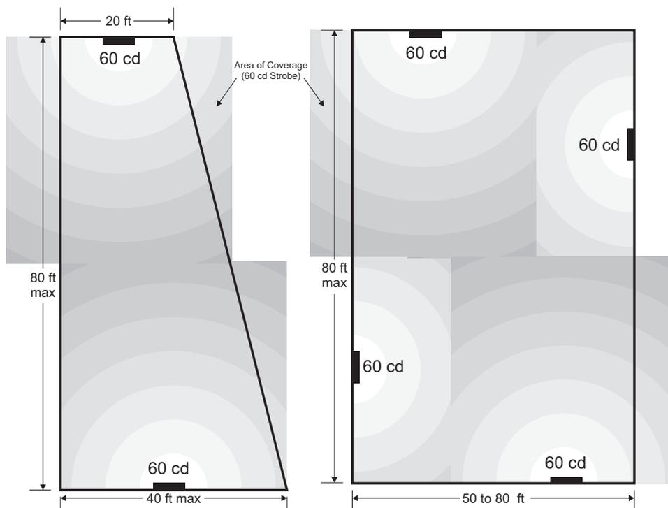
Note: Where more than one strobe is placed in any single field of view, only devices that flash in synchronization should be used. Failing to do so can result in aggregate flash rates high enough to trigger photoepileptic seizures among a portion of the population.
