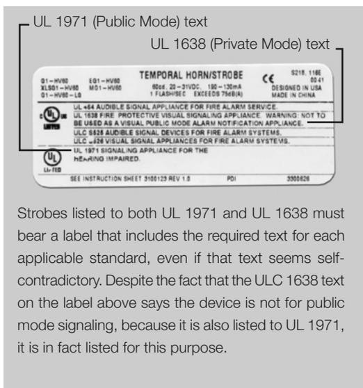
Strobes listed to both UL 1971 and UL 1638 must bear a label that includes the required text for each applicable standard, even if that text seems self-contradictory. Despite the fact that the ULC 1638 text on the label above says the device is not for public mode signaling, because it is also listed to UL 1971, it is in fact listed for this purpose.
