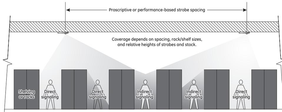
Adding the cd values in each example to arrive at a total candela output for a room of this size reveals that the two configurations are identical. This will result in more or less equal power requirements. But a word with your local supplier may reveal that the cost of four 135 cd strobes is significantly higher than the cost of nine standard 60 cd devices, even when the extra wiring is taken into account.
