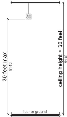
**702.3.4 Spacing Allocation and Minimum Intensity.** Spacing and minimum effective intensity for appliances shall comply with 702.3.4.
